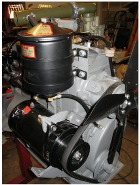
Finally with the generator around the fan belt, and arm holding the generator in place, you want to try and add the spring on the arm. Tighten the nut on the arm to generator and verify you have very little play in the fan belt. These wide belts don't need much tension. You should be able to deflect the belt about 1/2" with moderate finger pressure. Excessive tension is hard on water pump bearings. (tip from Pete Silfven) <br><br>Nice picture provided by Mike Strohlein
