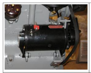
Here is the backside of the generator installed. You can adjust the arm based on where your generator lines up, and the pressure on the fan belt.<br><br>Nice picture provided by Mike Strohlein
