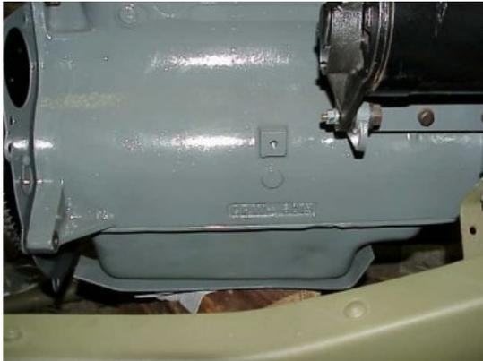
Whether you have many miles on your engine or a fresh rebuild, you may be faced with replacing your rear main seal. You will not have excessive oil leaking around the front of the bell housing. Don't be confused by thick gear oil from your transmission. Anyway, first remove the oil pan.
