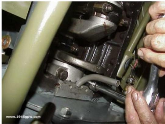
Put the bottom half of the seal in the cap and slide the main cap back into position and tighten down. You should see a little excess gasket sealer come out if you applied any. If so, wipe it down.
