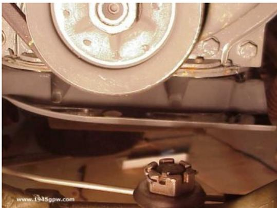
Pan and pulley are on, wait a bit for sealer to harden up. Install your oil back into the engine, check for leaks on the pan. If all looks good, start the engine up and see if the rear main seal leaks anymore.
