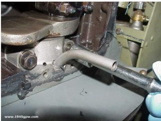
Follow the crank shaft towards the transmission bellhousing. You want to remove the main cap. Two bolts holding the drive shaft in position
