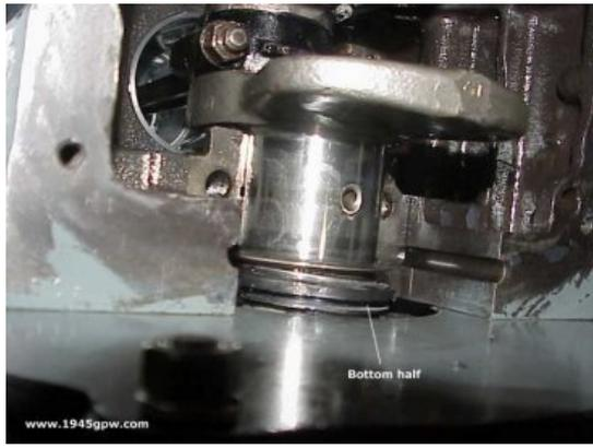
Oil your seal down and slide it into position on the top half. If that goes well, you don't have to pull the engine and drop the crank. If it doesn't then you will need to drop the crank out of the pan a bit. (Pete Silfven tip) If the top half is difficult to install, rotating the crank while installing it will help get it in.
