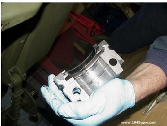
When the bolts have been removed, slide the main cap out and inspect. There should be to rubber wick type packing on each side. Remove these. Inspect the cap and the main seal that should fall with it
