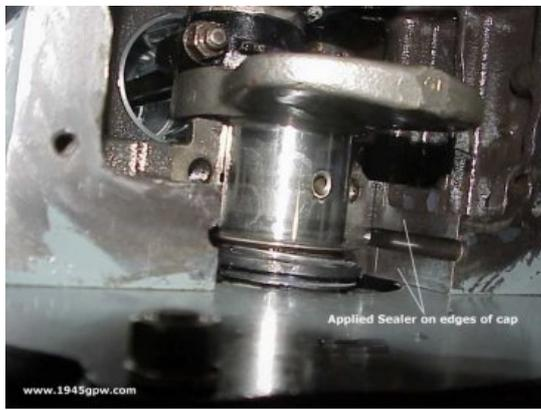
Before installing the main cap back in, we apply a little Right Stuff gasket sealer.
