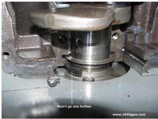
Here is the trick if you can do it. The issue with the crank in place is it holds the top half of the rear main in place. Try and pull it out with needle nose pliers, or screw in a metal screw and try pulling it out.
