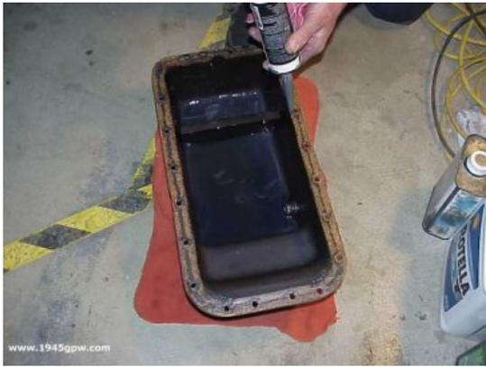
Clean off the oil pan of the old gasket, and replace with a new gasket. Apply a little gasket sealer on the side that will be applied to the block. Then install.
