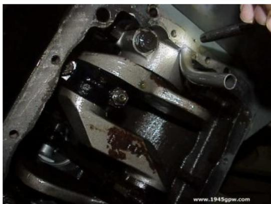
Prior to placing the oil pan back on, clean off the old gasket and sealer on the block with a putty knife. Using solvent, make sure the hole area for the oil pan is clean and clear of debris.
