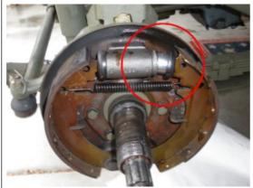
Test Wheel Cylinders with Drums
