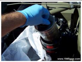
Here I will put a couple baggies from the grocery store to immediately transfer the old oil filter into it. Trying to avoid spilling oil all over the engine and ground.
