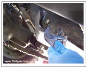
Remove the oil pan plug by turning the plug counter clock-wise.
