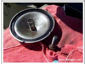
New seal installed, now place the lid on the filter housing and tighten up.
