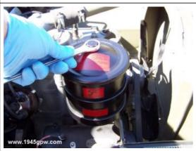
Prior to installing the lid you should inspect the copper washer and replace if needed. These are pretty weak so replacing them is common
