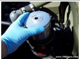
Install the new filter into the filter housing. You can use the following Oil Filter elements. NAPA 1100, Purolator PD51R, WIX 51100, AC P115 You can find it here at Napa Auto
