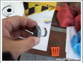
I place pipe tape around the plug thread to help stop leaking. I have drips that come from this plug, so I add thread tape to help stop that from that area.
