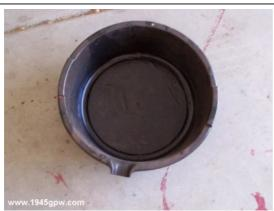
You will need to a have a catch pan of some sort. Here I have an oil catch pan which will hold about a gallon and half of fluid
