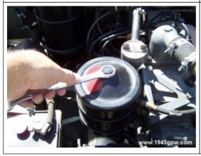
Remove the oil filter housing lid. Unscrew counter clockwise.
