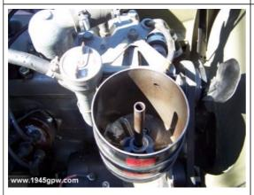
Here you see the filter housing is empty and there is no particles in the housing.
