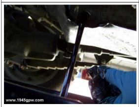
Let the oil drain into the pan. While this is draining, I will head over to the oil fitter and prepare to remove it.
