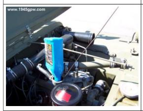
The TM's call for 30 weight oil. I use 10w30. Stay away from the higher viscosity oils like 20w50. Add Oil checking the amount on the dipstick. Its a little over 4 quarts.
