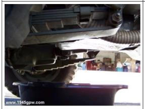
Place the oil catch pan under the oil plug. It gets kind of windy here so I adjust the pan based on the wind and how I estimate it blowing the oil around.
