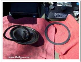
Remove the old oil filter seal from the lid, and prepare the new seal. I will coat the new seal with a little oil before placing on the lid.
