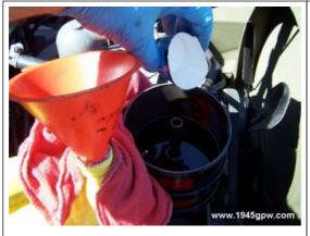
There is an oil plug on some filter housings down at the bottom. If I drain from this drain plug I will get oil all over the engine and ground. So I remove it by dipping a small cup into the housing and set my drain container right next to it. and start scooping out the oil. I will do this all the way down to the bottom and then wipe out the filter housing and check for debris.
