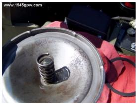
Clean the lid around the edges thorougly before placing the new seal on. Crud builds up on the edges of the lid, so be sure to wipe it down clean before installing the new seal.
