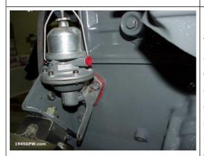
Insert the fuel pump and line up the two bolts to the block. You may need a swivel socket to reach the left bolt on the fuel pump. If you applied gasket sealer, then wipe off any excess. Keep the pump rotated slightly counterclockwise so you don't have to work against spring tension while starting the front bolt. After it's started, swing the pump clockwise so the rear hole matches up and install the rear bolt
