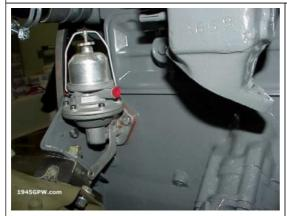
Installing a fuel pump is easy if you have everything removed and out of the way. If not, one of the two bolts will give you havoc because its difficult to reach.
