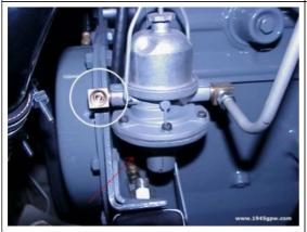
Before you install your fuel pump look at what is going to get in the way first. The top brass fitting MUST be installed on your pump first, because you will not have any room to spin it once your pump is tighted down. The other issue is how to reach the bolt on the left that holds the pump to the block.
