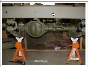
Installing propeller shafts is not a difficult job. To start with, make sure your jeep is off the ground and the transmission. Place your transfer case gears to engage in 4W high or low, otherwise when you try and tighten your u-bolts the axle will want to spin.
