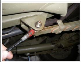
Next, scoot out from the jeep and hit the back wheel spring bolt. After this one is done, set the grease gun aside and check the fluids on the transmission
