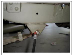
Move around the passenger back wheel and hit the rear spring shackle bolt.
