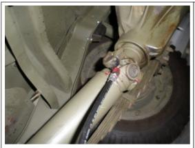
While under the jeep, shift to the back axle shaft and hit the zerk on the universal joint (if you can). If the zerk is not in a position, you will need to rotate by moving the jeep forward or backwards.
