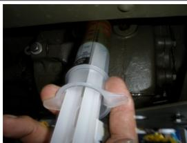
And I squirt the gear oil into the transfer case. With this device it takes about 5-6 fills to top off. But, no mess.
