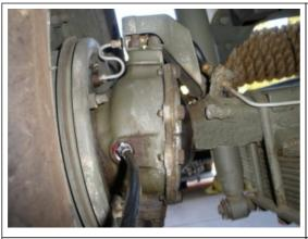
Next, unscrew the front axle universal plug behind the driver wheel. Stick you pinky finger into the axle housing and see if you can feel grease. Most likely not, as the grease settles at bottom. I will give 5-10 squirts into the drum.
