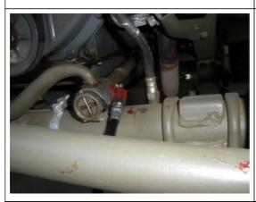
Behind the bell crank for steering is the drag link for steering. You can hit the front fitting while you are here. And get the back fitting when we are under the driver side.
