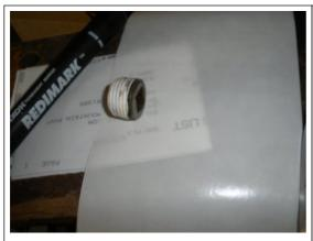
I will tape up all of the plugs around the transmission/transfer case to avoid dripping. If you changed the fluid then tighten this one back up and we will fill when we are on the passenger side.
