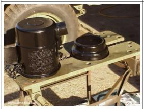
First you need to clean out your oil bath air filter unit. Remove all oil, and clean well with a degreaser.
