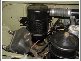
One common modification to your WWII jeep configuration is to change the Oil Bath air filter to a more modern efficient Dry air filter. Here we show you the common parts needed to make this change. Note: this configuration will work with non-pancake air filters from early 1942 to 1945.
