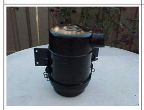
Place the Air Filter housing over the items you just installed and fasten the clips to the unit. Its now ready to use!
