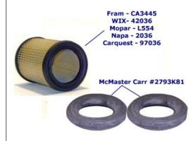
You need three parts, (1) Air Filter, (2) Rubber Gaskets. First you can get the air filter #2036 for about \$8 from Napa. Then you need Sponge Rubber rings 3" x 4" x 3/4" from McMaster Carr #2793K81 which are about \$3 each.
