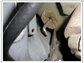
Now move back to the other side of the firewall and see that the lip of the boot is properly pulled through. You may need to use some needle nose pliers to help pull part of the lip around evenly.
