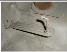
From the opposite side of the firewall (near driver seat), pull back on the foot pedal. It will lie as shown here.
