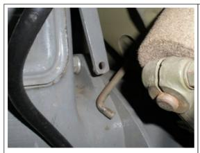
With the cotter pin out, push the gas pedal arm out so it lies freely.
