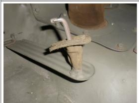
Place the boot over the gas pedal arm as shown
