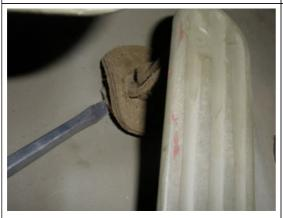
With a screw driver, carefully push the edges on the back of the boot through the firewall hole. Be careful not to puncture the boot. Move your screw driver around the boot until you believe the back lip of the boot has been pushed through
