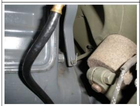
In picture, you see the linkage is easy to get to. Removing the cotter pin releases the Gas Pedal arm and it is an easy install. But in this picture, the driver fender was removed as well as the manifold on the engine.
