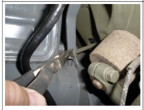
To release the gas pedal arm, remove the cotter pin from the linkage. Use a needle nose plier to crimp and pull the pin out.
