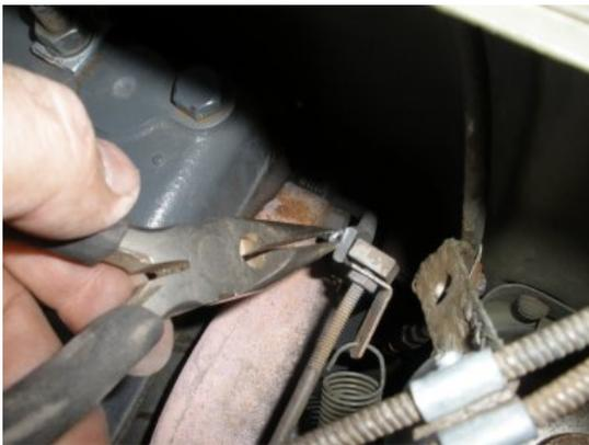
Remove the cotter pin from the gas pedal armature. Note: it is a good habit to replace cotter pins after removing them.
