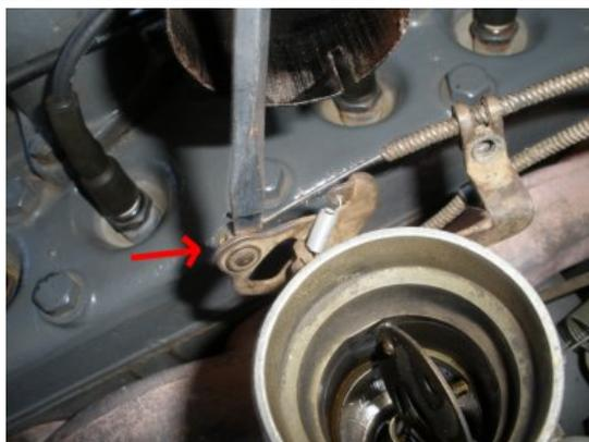
Loosen the throttle screw.
