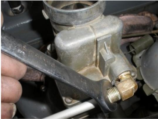
Next, line up the fuel line to the carburetor and tighten the connection.
