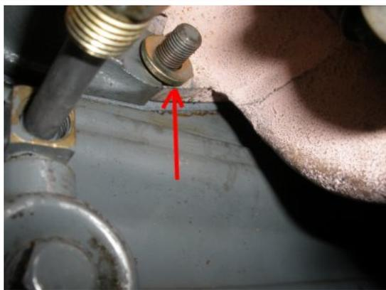
Just a note, be sure you have the correct washer on the two piece connections under the manifold (where intake and exhaust come together). Tighten all the nuts on to the manifold, all seven!
