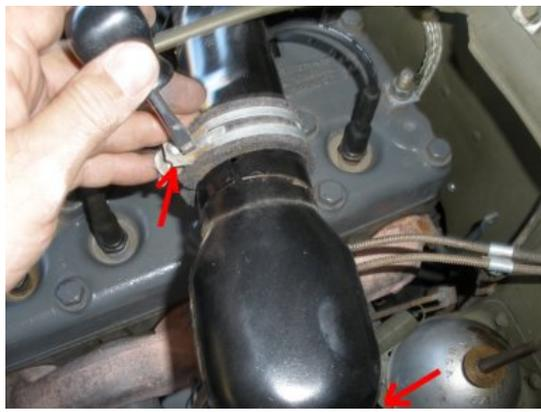
Next, loosen the clamp on the air horn seal. Move it down the tub once loosened. In addition, loosen the air horn clamp and remove the air horn from the top of the carbureator.
