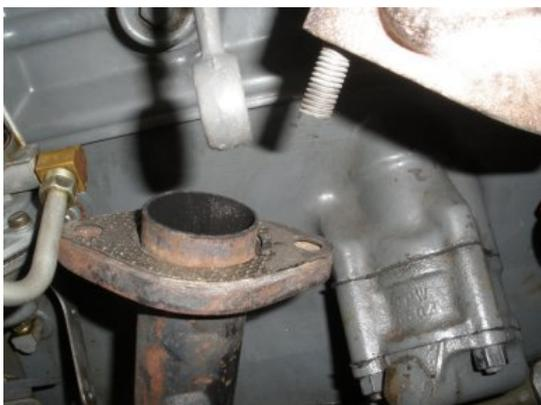
Disconnect the Exhaust flex pipe from the manifold. Note: watch for the gasket.
