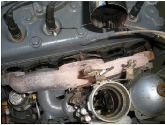
At this point, tug on the manifold a bit and it should separate from the block. It is heavy so it might take a decent tug. Try not to strip the bolts on the block on the way out.
