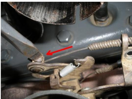
Install the throttle line back into the insert and tighten the screw down.
