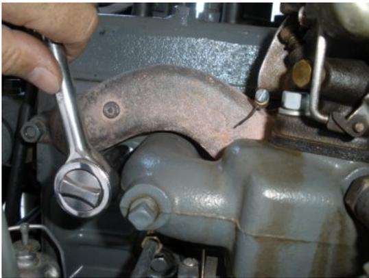
Locate each of the nuts on the intake/exhaust manifolds, and remove the bolts.
