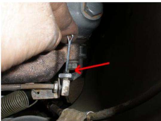
Install a new cotter pin to the gas pedal linkage. Insert and separate the ends of the new cotter pin with needle nose pliers if needed.
