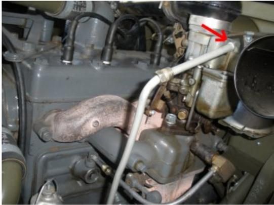
Remove the Fuel line from the carburetor
