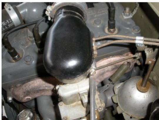
Now install the air horn back on top of the carburetor. Fit the horn into the air tub and clamp the base of the air horn to the top of the carburetor.
