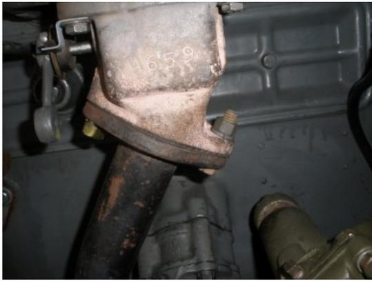
Add a new exhaust gasket to the exhaust flex pipe and tighten the bolts into the bottom of the manifold.
