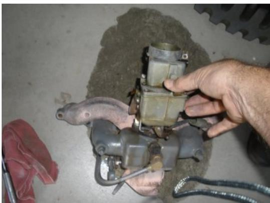
Note: the carburetor is most like still filled with fuel, so if your not careful you will spill the fuel all over the place. This is an example of what not to do :(
