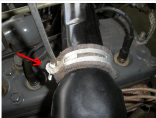
Finally, pull your seal back from the air horn back over where the two peices meet, and tighten down. You have now reinstalled your manifold!
