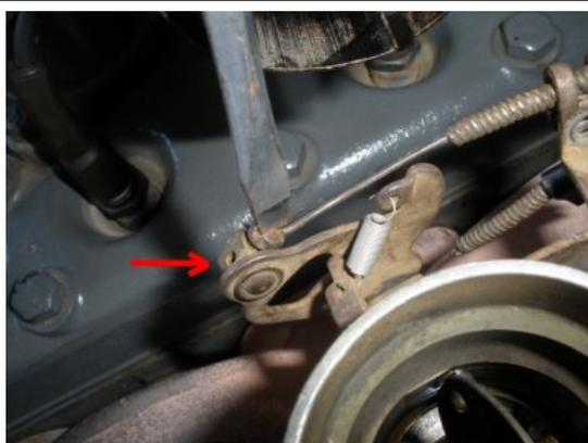
The throttle cable will slip out of the screw holder.
