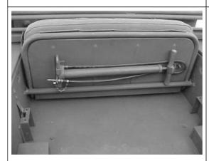
The pump will fit snugly under the rear seat with the clamp on the handle, and the air chuck nozzle fitting through the lower bracket.
