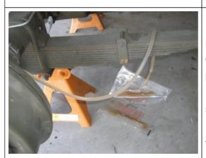
Now with all the speedbleeders now in the wheel cylinders and tightened down, move back to the Rear passenger side, and attach the tube retainer in the line. Loosen the speedbleeder about 1/4 - 1/2 a turn. Pump the brakes slowly about 4 times. The speedbleeders will open pushing the brake fluid out, and close when the pedal is retreating. Here you see the line is full and the fluid being push out with each brake stroke.
