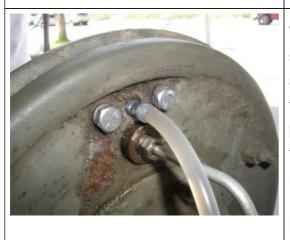
With a closer examination, you can see that the air in the fluid has already been pushed out. Now, tighten the bleeder (clockwise) and pinch the tube off at the bleeder and the fluid will flow down into the retainer bag.
